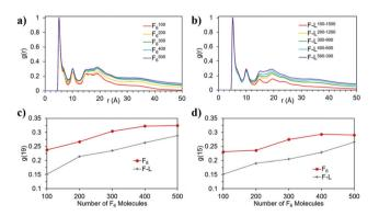
Fig. 4 Normalized RDF of the F<sub>6</sub> molecules in the (a) control and (b) co-assembly simulation; and evolution of the RDF intensity, q(r), at (c) r = 19 and (d) r = 15 for the control (F<sub>6</sub>) and co-assembly (F-L) systems as a function of the number of F<sub>6</sub> molecules.
