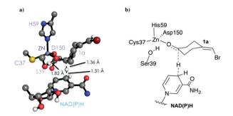
Scheme 2 DFT optimized TS structure for the hydride transfer step. For visualization purposes, non-polar hydrogen atoms are hidden.
