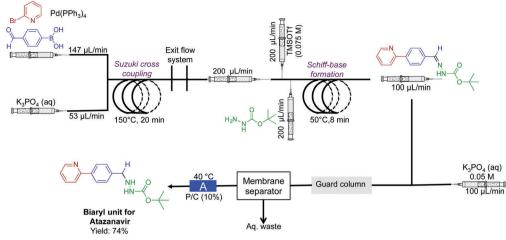
Fig. 10 Continuous-flow synthesis of the biaryl unit for the API atazanavir. A three-step sequence afforded the bi-aryl motif in 75% yield.<sup>32</sup> The reactor labeled A is the H-cube pro.
