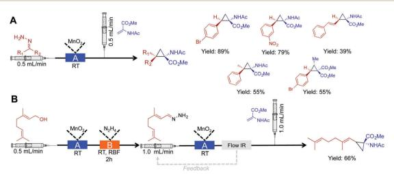
Fig. 7 Continuous-flow synthesis of cyclopropane rings. (A) A two-step process converts hydrazine into cyclopropane rings via the diazo species.<sup>28</sup> (B) Extending this to a three-step procedure allows the conversion of alcohols to cyclopropane rings. In both the schematics: Reactor A - column packed with manganese dioxide, and Reactor B - round bottom flask containing 1.05 eq. N<sub>2</sub>H<sub>4</sub>.
