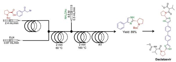
Continuous-flow synthesis of an imidazole fragment en route to the synthesis of Daclatasvir.<sup>50</sup>
