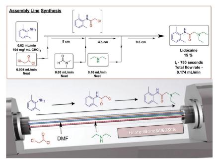
Fig. 25 Continuous-flow synthesis of lidocaine using an assembly line inspired process contained within dynamic thin films using a vortex fluidic device.<sup>50</sup> Reproduced from ref. 50 with permission of Wiley, copyright 2017.
