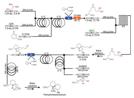
Fig. 16 Semi continuous-flow synthesis of perhydrohistrionicotoxin. In this example, seven out of the eleven steps were mediated in continuous flow.<sup>37</sup>
