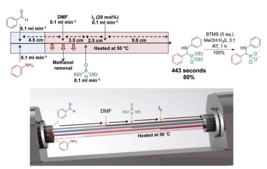
Fig. 11 Continuous-flow synthesis of an α-aminophosphonate using dynamic thin films in an assembly line fashion.<sup>31</sup> This assembly line inspired approach synthesized an α-aminophosphonate in 80% yield for a seven min residence time. Reproduced from ref. 31 with permission of Wiley, copyright 2017.
