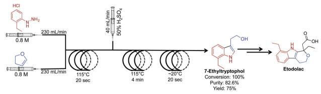
**Fig. 12** Continuous-flow synthesis of intermediate API 7-ethyltryptophol in the synthesis of etodolac. The three-step process produced 7-ethyltryptophol in 75% yield compared to only 45% in the batch process.<sup>33</sup>
