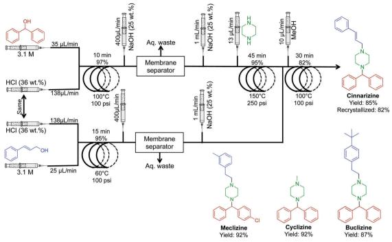
Fig. 22 Continuous-flow synthesis of cinnarizine, maclizine, cyclizine and buclizine. Four transformations convert the respective alcohols into APIs in good yields.48
