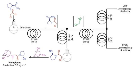
Fig. 13 Continuous-flow synthesis of the intermediate for API vildagliptin. Combining two synthetic steps into a semi-continuous flow system produced the key intermediate for this API at  $4.8 \text{ kg h L}^{-1.34}$
