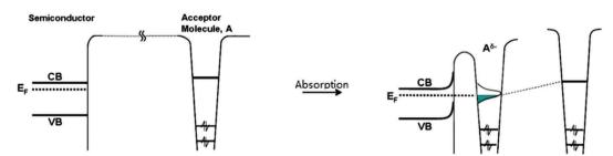
Fig. 4 Schematic diagram shows the adsorption of an acceptor molecule (A) onto a semiconductor surface. Modified from ref. 7 with permission of the American Chemical Society
