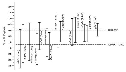
Band positions of various semiconductors with respect to the redox potentials of water splitting at pH = 0
