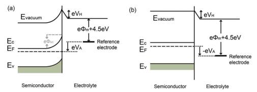
Fig. 5 Effect of applying a bias voltage  $(V_A)$  to an n-type semiconductor photoelectrode.  $V_H$  is the potential drop across the Helmholtz layer.  $\Phi_m$  is the work function of the metal.  $\Phi_{sc}$  is the potential drop across the space charge region. Reproduced from ref. 3 with permission of Springer Science+Business Media, LLC.
