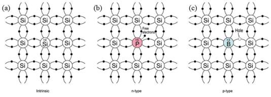
Schematic bond representation for (a) intrinsic silicon; (b) n-type silicon doped with phosphorus and (c) p-type silicon doped with boron.
