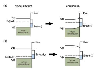
Fig. 3 Schematic illustration of surface-state induced band bending: (a) disequilibrium and equilibrium between the bulk and the surface for an n-type semiconductor; (b) disequilibrium and equilibrium between the bulk and the surface for a p-type semiconductor; modified from ref. 7 with permission from the American Chemical Society
