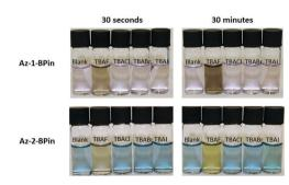
Fig. 3 Photograph of test solutions of Az-1-Bpin and Az-2-Bpin upon exposure to tetra-n-butylammonium halides in THF. In each solution, [analyte] = 180  $\mu$ M, which for TBAF corresponds to 3.4 mg L<sup>-1</sup> of fluoride anion. (For absorption spectra, see Fig. S1 in the ESI†).
