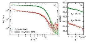
Fig. 4 (a) Small-angle X-ray scattering data and best fits (black-dashed lines) to the model described in the text of CTAB/TBAS before (green) and after (red) the incorporation of the **Az-1-Bpin** indicator (b) Guinier plot.
