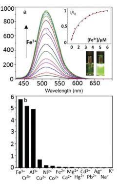
Fig. 2 (a) Steady-state single photon fluorescence spectroscopy ( $\lambda_{\rm ex}$  = 403 nm) of **TNP** (1  $\mu$ M) in ethanol–water (80 : 20, v/v) with a buffer solution of HEPES (10 mM, pH = 7.4) in the presence of different concentrations of aqueous metal ions. Inset: Fluorescence intensity at 515 nm of **TNP** as a function of aqueous Fe<sup>3+</sup> concentration. (b) Fluorescence intensity change of **TNP** (1  $\mu$ M) in the presence of metal ions (10  $\mu$ M).
