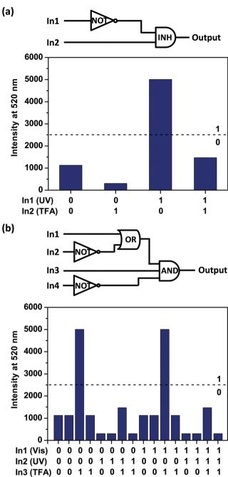
Fig. 3 (a) Schematic diagram of aqueous INH logic gate with two inputs: In1 (UV light), In2 (TFA) and a single output:  $I_{520}$  (the normalized fluorescence intensity at 520 nm). The actual output values are shown below the diagram. (b) A more complicated logic circuit designed with four inputs: In1 (visible light), In2 (UV light), In3 (TFA) and In4 (TEA), and a single output:  $I_{520}$  (the normalized fluorescence intensity at 520 nm). The actual output values are shown below the diagram.
