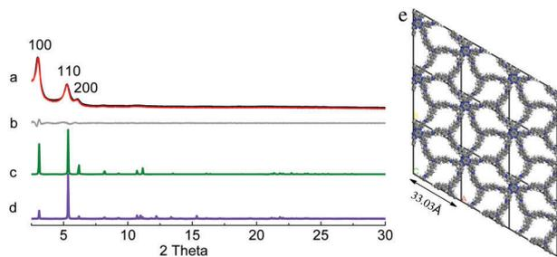
Fig. 2 (a) Experimental (black) and refined (red) PXRD patterns of **HAT-NTBCA-COF**, (b) difference plot between the experimental and refined PXRD patterns, and simulated PXRD patterns of the COF with (c) AA and (d) AB stacking, and (e) the unit cell structure of **HAT-NTBCA-COF** in AA stacking.
