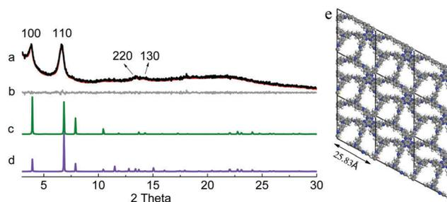
Fig. 1 (a) Experimental (black) and refined (red) PXRD patterns of **HAT-NTBA-COF**, (b) difference plot between the experimental and refined PXRD patterns, and simulated PXRD patterns of the COF with (c) AA and (d) AB stacking, and (e) the unit cell structure of **HAT-NTBA-COF** in AA stacking.
