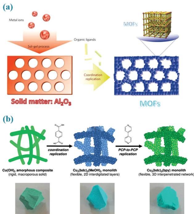
Fig. 4 (a) Coordination replication of  $\text{Al}_2\text{O}_3$  with honeycomb patterns to a more stable aluminium naphthalene dicarboxylate framework. Reprinted from ref. 61 with permission from Nature Publishing Group. (b) Two step coordination replication of the  $\text{Cu}(\text{OH})_2$ -polyacrylamide composite to 2D layered frameworks and 3D networks. Reprinted from ref. 45 with permission from the Royal Society of Chemistry.
