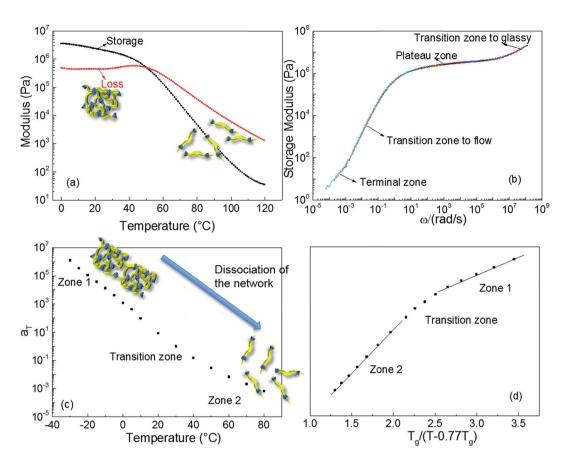
Fig. 2 The rheological behaviour of polyurethane 1. (a) Temperature sweep at 5 Hz; (b) master curve at a reference temperature of 30 °C, different colours corresponding to different temperatures; (c) time–temperature shift factor  $a_T$  of polyurethane 1 as a function of temperature; (d) plot of  $a_T$  for polyurethane 1 as a function of temperature normalized to  $T_q$ .
