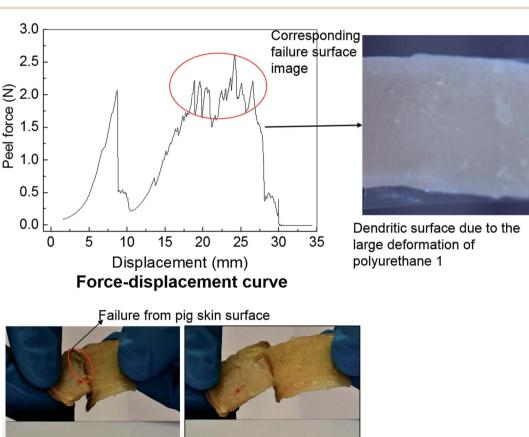
Failure from polyurethane 1
