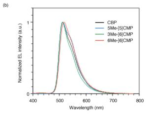
Fig. 5 Performance of the single-layer OLED. (a) External quantum efficiency of the single-layer OLED plotted against the current density. See Fig. 1a for the device architecture. (b) Electroluminescence spectra at a current density of  $0.1 \, \text{mA cm}^{-2}$ .
