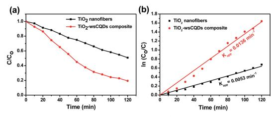
Fig. 7 (a) Photocatalytic degradation of MB in presence of  $TiO_2$  nanofibers and  $TiO_2$ -wsCQDs composite under UV light irradiation and (b) photocatalytic reaction kinetics of MB degradation in presence of  $TiO_2$  nanofibers and  $TiO_2$ -wsCQDs composite.
