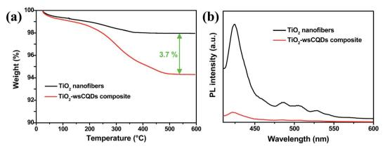
Fig. 6 (a) TGA graph of  $TiO_2$  solid nanofibers and  $TiO_2$ -wsCQDs composite and (b) PL spectra of  $TiO_2$  nanofibers and  $TiO_2$ -wsCQDs composite.
