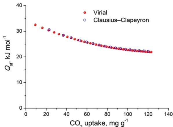
Fig. 6  $CO_2$  isosteric heat of adsorption ( $Q_{st}$ ) in Cu-PEIP as a function of surface coverage, calculated from a virial-type analysis. The corresponding Clausius–Clapeyron calculation is also shown, for comparison.
