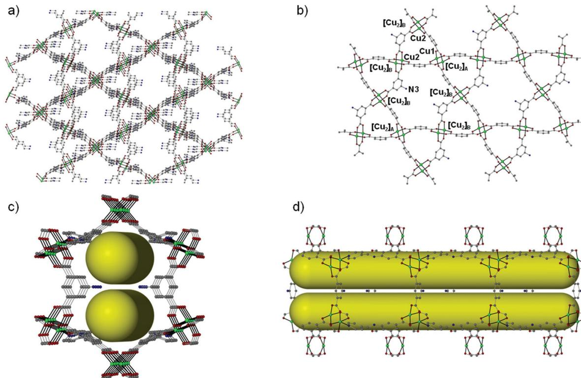
**Fig. 2** Representations of (a) the 3D framework along the *a* axis, (b) the (3-6-3-6) semi-regular net (augmented Kagomé lattice: *kgm-a*), (c) the compartmentalized hexagonal channels along the *a* axis and (d) the compartmentalized channel projected along the *a* axis for complex **Cu-PEIP**. Colour code: Cu green, O red, N blue, C gray. H atoms are omitted for clarity.
