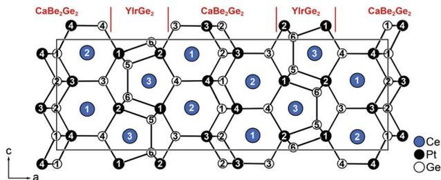
**Fig. 3** Extended unit cell of the commensurate supercell structure ( $Pnma$ ,  $a = 2618.26(14)$ ,  $b = 441.33(2)$  and  $c = 882.34(2)$  pm) of  $Ce_3Pt_4Ge_6$ . The  $YrGe_2$  and  $CaBe_2Ge_2$  type parts are labelled. Ce atoms are depicted as blue, Pt atoms as black and Ge atoms as open white circles.
