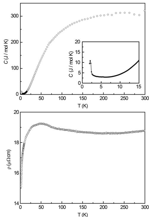
**Fig. 7** Physical properties of  $\text{Ce}_3\text{Pt}_4\text{Ge}_6$ : (top) Heat capacity measurement in the temperature range of 1.9–300 K, the inset shows the low temperature region between 1.9–15 K, indicating a  $\lambda$ -shaped anomaly; (bottom) temperature dependent electrical resistivity  $\rho$ .
