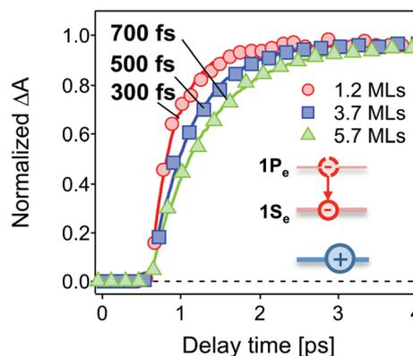
**Fig. 4** Normalized initial build-up kinetics of  $1S_e1S_{3/2}$  in the CdSe core capped with 1.2 MLs (red circles), 3.7 MLs (blue squares) and 5.7 MLs (green triangles) of the CdS shell. The build-up time constants are derived by a single exponential fitting (solid lines), showing an increase with increasing shell thickness. The excitation wavelength was 400 nm. Inset: the  $1P_e$  hot electron relaxes to the  $1S_e$  state.
