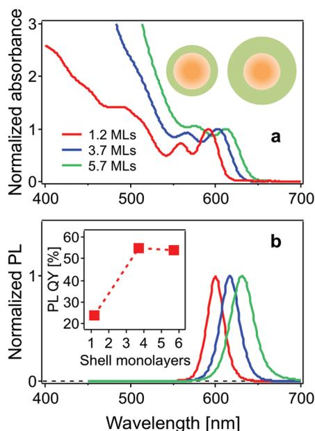
**Fig. 1** (a) Normalized absorption and (b) PL spectra of CdSe/CdS QDs with 1.2, 3.7, and 5.7 monolayers of the CdS shell in chloroform. Inset in (a): a schematic diagram showing the CdSe/CdS core/shell structure with thin (left) and thick (right) shell. Inset in (b): the PL quantum yield as a function of CdS shell thickness.
