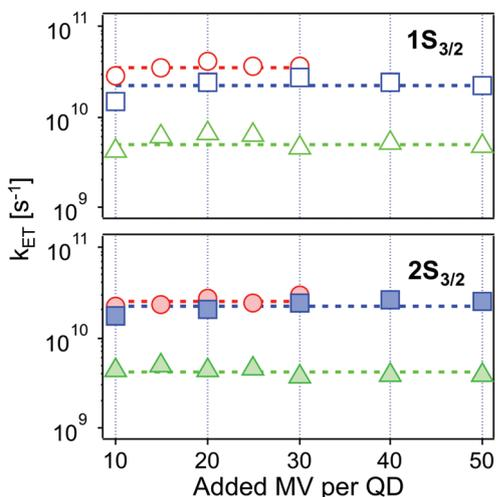
**Fig. 6** Intrinsic ET rates from  $1S_e1S_{3/2}$  (top, open symbols) and  $1S_e2S_{3/2}$  (bottom, solid symbols) state in CdSe/1.2CdS (red circles), CdSe/3.7CdS (blue squares) and CdSe/5.7CdS (green triangles) derived from eqn (4), as a function of added  $MV^{2+}$ . Dashed lines refer to the averaged ET rates. The experimental conditions were kept identical at each molar ratio for each batch of QD- $MV^{2+}$  complex.
