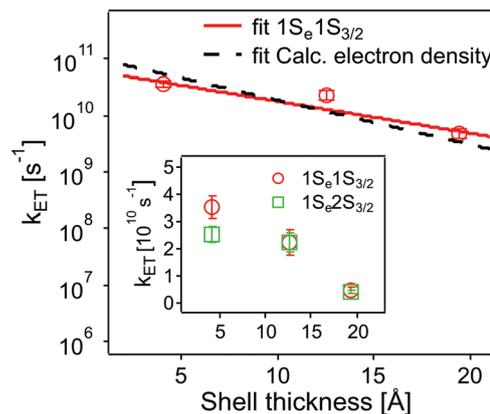
**Fig. 7** Dependence of intrinsic ET rates  $k_{ET1}$  from  $1S_e1S_{3/2}$  (red circles) and  $k_{ET2}$  from  $1S_e2S_{3/2}$  (inset, green squares) in QD- $MV^{2+}$  complexes on CdS shell thickness. Error bars indicate the calculated standard deviations in averaging the ET rates. Also shown is the calculated electron density (black dashed line) with different shell thickness (see text and ESI†). For comparison, the electron density is scaled to the measured ET rate.
