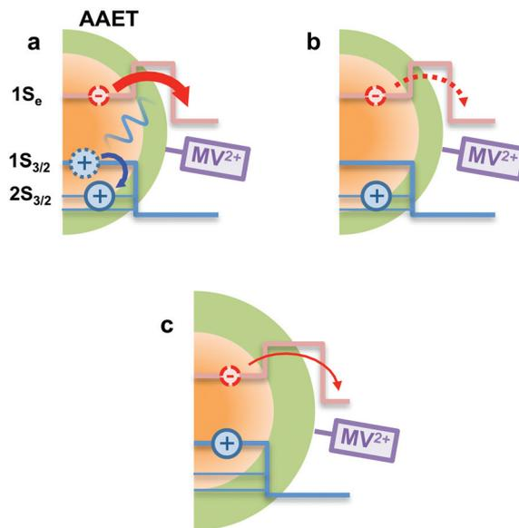
**Fig. 8** Schematic illustration of the AAET process. (a): In the AAET process, electron transfer to  $MV^{2+}$  is accompanied by the excitation of the  $1S_{3/2}$  hole to higher levels. (b): The Auger process lacks the  $1S_{3/2}$  to  $2S_{3/2}$  hole transition, leading to inefficient AAET. (c): With thick shell, the Auger-assisted channel is cut off due to the weak electron–hole coupling.
