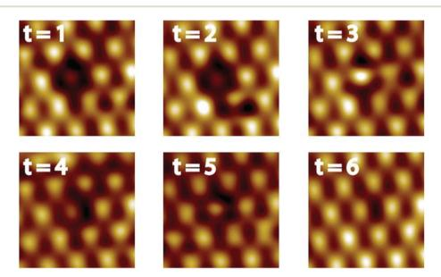
Fig. 6 High-resolution UHV-STM images of Pt-Pt<sub>3</sub>Ti (2.1 nm × 2.1 nm) showing the healing process of a defect by restructuring (T = 77 K). Time difference between two following STM images:  $\Delta t = 170 \text{ s}$  (0.94 V; 0.08 nA, low pass filtered).
