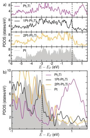
Fig. 4 (a) Total d-PDOS used to calculate the d-band centers ( $\varepsilon_{\rm d}$ ) for Pt<sub>3</sub>Ti, Pt-Pt<sub>3</sub>Ti, 2Pt-Pt<sub>3</sub>Ti and Pt(111)-substrates (see Table 1). (b) Comparison of the total d-PDOS of the simulated terminations in the energy range around  $E_{\rm F}$ .
