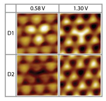
Fig. 5 Two different characteristic surface defects on S1 (Pt-Pt<sub>3</sub>Ti), D1 and D2 (0.58 V, 0.48 nA; 1.30 V, 0.11 nA; low pass filtered; 1.7 nm  $\times$ 1.7 nm).
