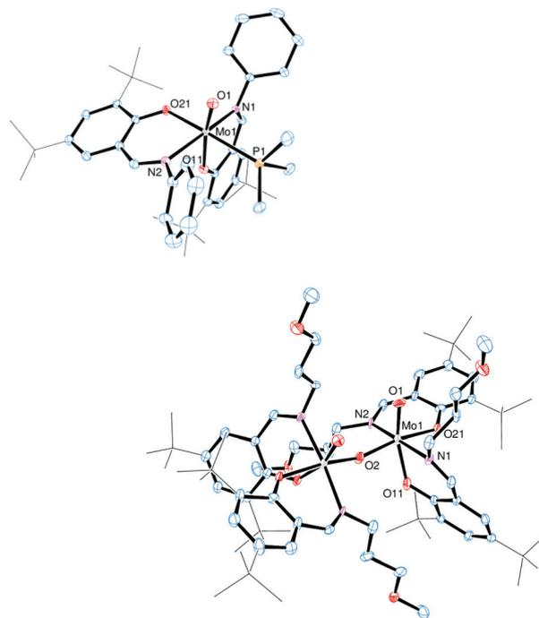
**Fig. 3** Molecular views (50% probability level) of **5** (top), and **6** (bottom); hydrogen atoms as well as solvent molecules are omitted for clarity, and *tert*-butyl substituents are depicted as a wireframe. For disordered fragments, only atoms with the higher site occupation factors are depicted. In complex **6**, only atoms in the asymmetric unit are labelled.
