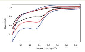
Fig. 1 Cyclic voltammetry of 2 at 25 mV  $s^{-1}$  (black), 100 mV  $s^{-1}$  (red), and 250 mV s<sup>-1</sup> (blue) in THF solution with 0.1 M [Bu<sub>4</sub>N][PF<sub>6</sub>] electrolyte. Glassy carbon working electrode, platinum counter electrode, Ag wire pseudo-reference electrode, 298 K.
