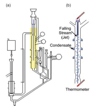
Fig. 1 (a) Hickman's falling-stream tensimeter apparatus designed in 1952 to measure evaporation coefficients. (b) Close-up view of the falling stream and condensate collection ports. Adapted with permission from K. C. D. Hickman and D. J. Trevoy, Ind. Eng. Chem., 1952, 44, 1882-1888. Copyright 1952 American Chemical Society.
