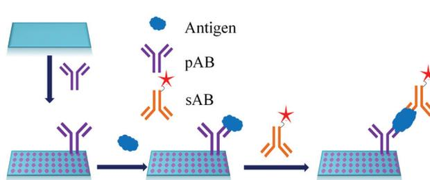
Fig. 16 Detection of PSA on the protein microarray.
