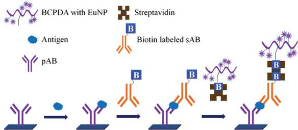
Fig. 13 Signal amplification for the detection of PSA.
