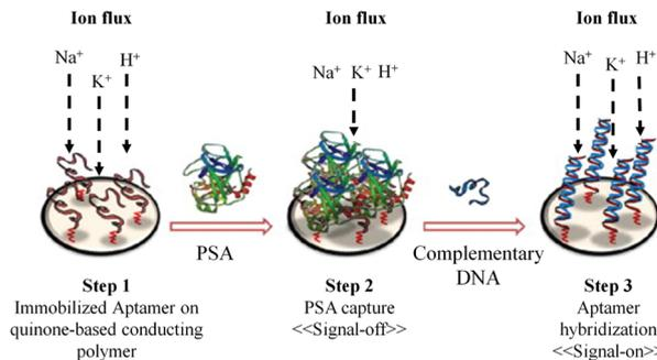
Fig. 7 Working principle for the “off-on” detection of PSA using an aptamer capture probe, followed by hybridization with a complementary sequence (adapted from *Biosens. Bioelectron.*, 2015, 15, 68, 49–54).
