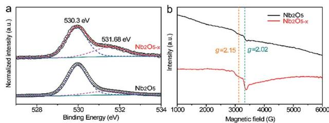
Fig. 2 (a) Normalized O 1s core-level XPS and (b) EPR spectra collected for Nb<sub>2</sub>O<sub>5</sub> and Nb<sub>2</sub>O<sub>5-x</sub> NPs films.
