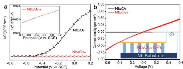
Fig. 3 (a) Mott-Schottky plots of Nb<sub>2</sub>O<sub>5</sub> and Nb<sub>2</sub>O<sub>5-x</sub> NPs films at a frequency of 1 kHz in the dark; (b) comparison of *I*-*V* curves of the samples; the inset is the schematic of the measurement.
