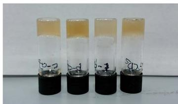
Fig. 4 Optimised ionic-liquid CD–Gel hybrid materials of composition 1 wt% **1a** in 500  $\mu\text{L}$  of CD solution at  $1 \text{ mg mL}^{-1}$  containing 2% BMIM-BF<sub>4</sub> (left-to-right c-CD, p-CD, t-CD and a-CD).
