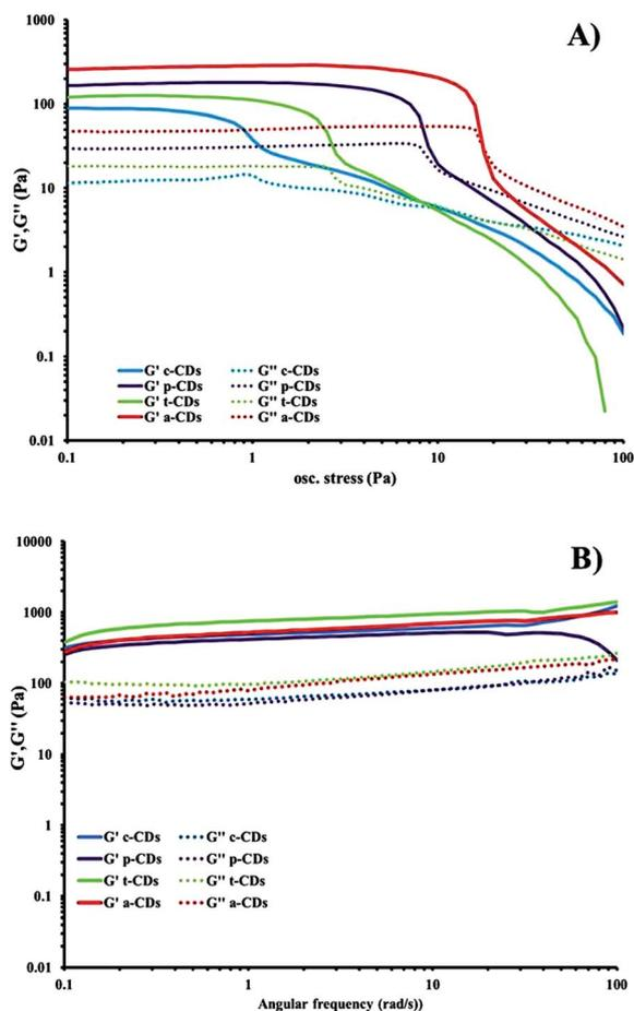
Fig. 5 (a) Stress sweep and (b) frequency-sweep rheology of dilute ionic-liquid CD–gel hybrid materials of composition 1 wt% **1a** in 500  $\mu\text{L}$  of CD solution at  $1 \text{ mg mL}^{-1}$  containing 2% BMIM-BF<sub>4</sub>.
