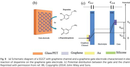
Fig. 9 (a) Schematic diagram of a SGGT with graphene channel and a graphene gate electrode characterized in electrolyte. (b) Electrochemical reaction of dopamine on the graphene gate electrode. (c) Potential distribution between the gate and the channel of a SGGT in electrolyte.
