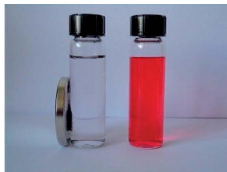
Fig. 8 Photograph of the fuchsine solution ( $20 \text{ mg L}^{-1}$ , right) and the solution after adsorption with the G/ $\text{Fe}_3\text{O}_4$  adsorbent for 1 h and separation with a magnet (left). Reproduced with permission from ref. 239.
