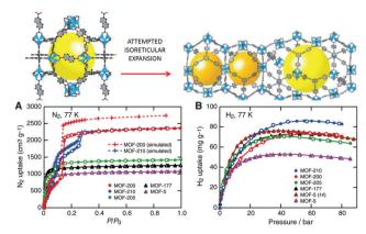
Fig. 11 (Up) The attempted isoreticular expansion of MOF-205 leads to MOF-210, and (bottom) the low-pressure N<sub>2</sub> isotherms (A) and high-pressure  $H_2$  isotherms at 77 K (B) of MOF-5, -177, -200, -205, and -210. Reprinted with permission from ref. 115. Copyright 2009. American Association for the Advancement of Science
