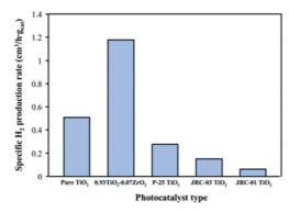
Fig. 15 The effect of the photocatalyst type on the specific H<sub>2</sub> production rate over the synthesised mesoporous-assembled pure TiO2 and 0.93TiO<sub>2</sub>-0.07ZrO<sub>2</sub> mixed oxide photocatalysts calcined at 500 °C when compared to commercial TiO2 photocatalysts (P25, JRC-01 Ishihara Sangyo Co., JRC-03 Ishihara Sangyo Co).
