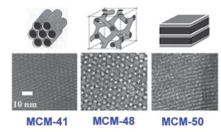
Fig. 1 Different structures of the M41S family: (top) surfactant supramolecular assemblies and (bottom) TEM images of the final materials. Reproduced from ref. 5. Copyright 2013, RSC.
