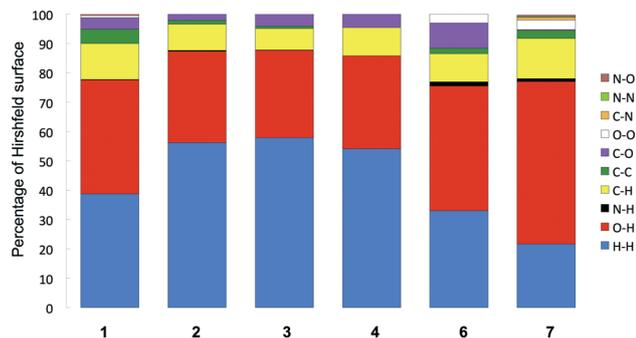
Fig. 3 The major contributions to the Hirshfeld surfaces in terms of closest atom–atom interactions for compounds 1–4 and the glycine derivative 6 and benzene-1,3,5-tricarboxamide 7, a rough first way to compare intermolecular interactions.
