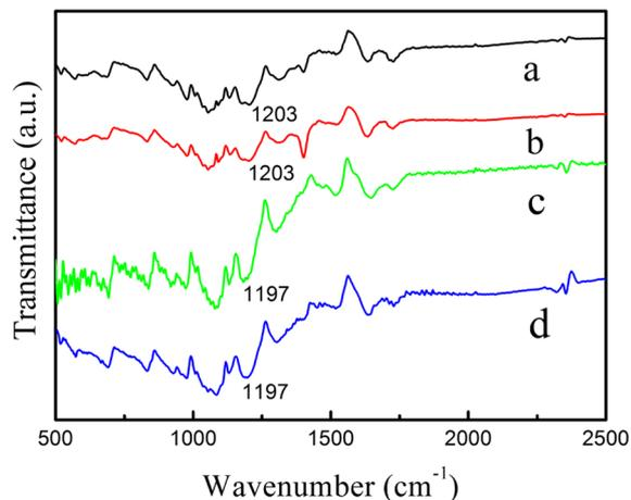
**Fig. 4** FT-IR spectra of prepared samples: (a) pure PEDOT:PSS, (b) PEDOT:PSS doped with DMSO, (c) SWCNTs/PEDOT:PSS layered nanostructure, (d) SWCNTs/PEDOT:PSS (doped with DMSO) layered nanostructure.
