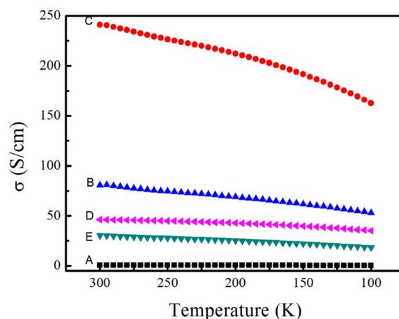
**Fig. 3** Temperature dependence of the electrical conductivity of the prepared samples: (A) pure PEDOT:PSS nanofilm, (B) SWCNTs/PEDOT:PSS layered nanostructure, (C) SWCNTs/PEDOT:PSS (doped with DMSO) layered nanostructure, (D) SWCNTs/PSS layered nanostructure, (E) SWCNTs/PVA layered nanostructure.
