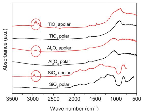
Fig. 2 FTIR absorption spectra of the used nanoparticles as received. Circles show the absorption at bands near the stretching vibration of hydrocarbon groups.<sup>26</sup>
