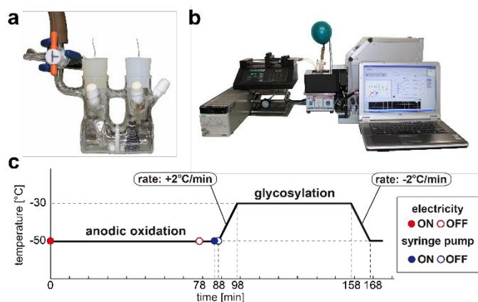
Fig. 3 Devices for automated electrochemical assembly. a) Divided electrolysis cell equipped with platinum plate cathode and carbon fibre anode. b) The 1st generation automated electrochemical synthesizer. c) Schedule of synthesizer for a single cycle.
