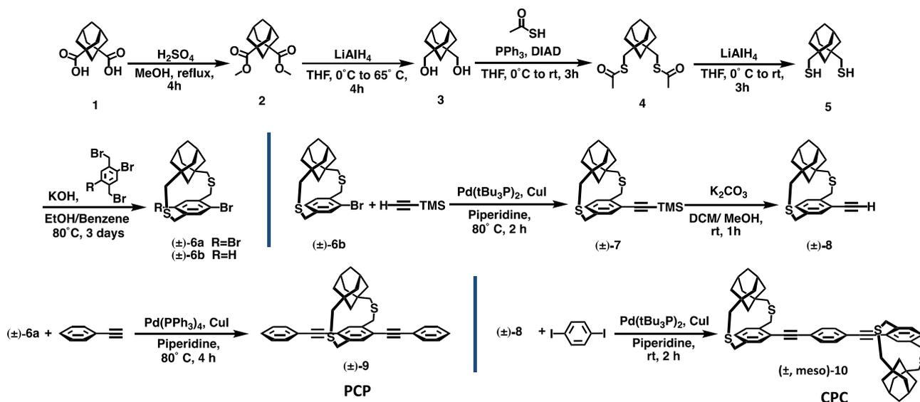
**Scheme 2.** Scheme for the synthesis of Donors ( $\pm$ )**9** (PCP) and ( $\pm$ , meso)-**10** (CPC) and their precursors. and linear trimers (PLP and LPL). The percentage of dopant ionization increased by 15 and 59% in the case of PCP and CPC respectively compared to that of the PPP. DFT calculations have shown that binding energy of DDQ with both CPC and PCP are the same and higher than that of
