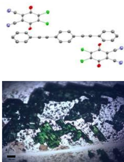
**Figure 7.** Single crystal X-ray thermal ellipsoid plots (top) and photograph (bottom) of PPP-DDQ charge transfer complex crystal. Thermal ellipsoids at 50% probability. Gray-C, red-O, green-Cl, blue-N (hydrogens are omitted for clarity). Scalebar is 100  $\mu\text{m}$ .
