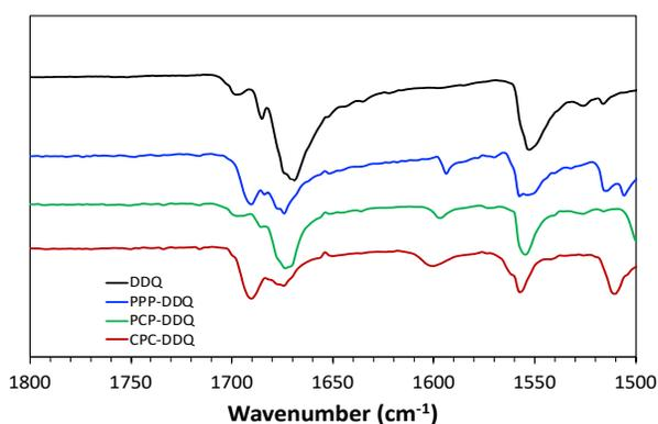
**Figure 2.** ATR-IR spectra of charge transfer complexes prepared from chloroform solution.
