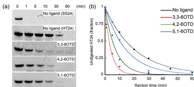
Fig. 2 (a) Time-course of remaining HT24 and SS24 (2  $\mu$ M) after S1 nuclease treatment in the presence of **1–3** (20  $\mu$ M). The gels were stained with SYBR-gold to visualize oligonucleotides. (b) Analysis of first-order kinetics of S1 nuclease reaction using remaining HT24 bands quantified by Image J.
