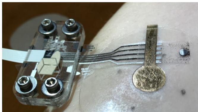
**Fig. 7** Human-subject testing on real skin including (a) diagram and (b) photographs of the test-setup.
