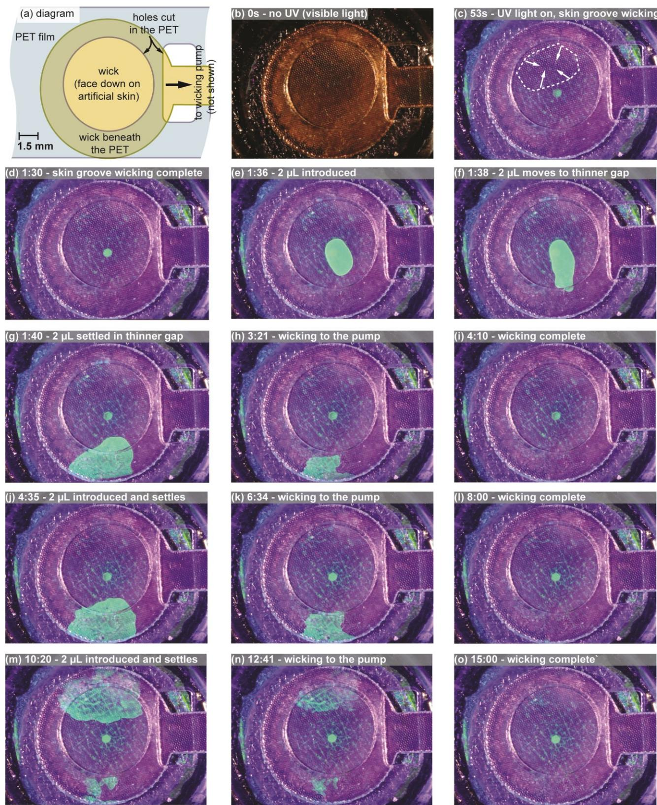
**Fig. 6** Testing on artificial skin including (a) diagram and (b)-(o) photographs labeled with time-stamps.
