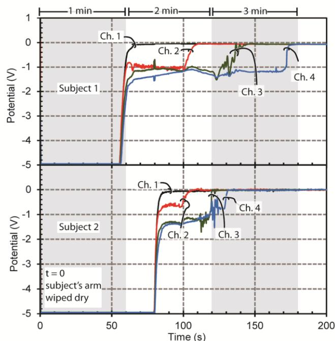
**Fig. 8** Electrode channel measurements vs. time for human-subject testing of (top) subject 1 and (bottom) subject 2. As each channel's potential changes to  $0$  V, it indicates that associated working electrode has been initially wetted and is fluidically coupled to the reference electrode via sweat.
