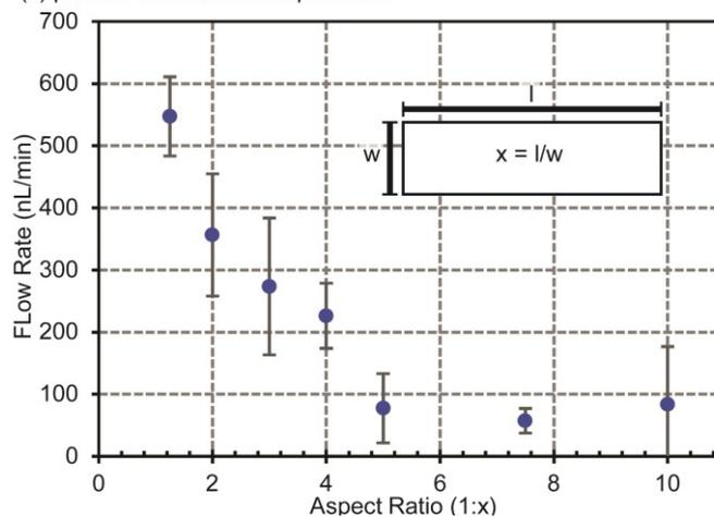
**Fig. 4** Setup for in-vitro characterization of flow rate through the hex wicks; **a)** test setup; **b)** capillary flow through the wick under the microscope; **c)** plot of flow rate vs. film aspect ratio.
