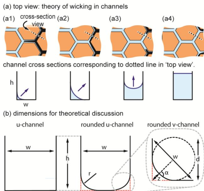
**Fig. 2** Theoretical framework of fluid flow in a hex wick **a)** top-view of hex wick with respective side-view of a channel filling representing the dotted-line shown in the top-views; **b)** dimensions governing fluid transport.
