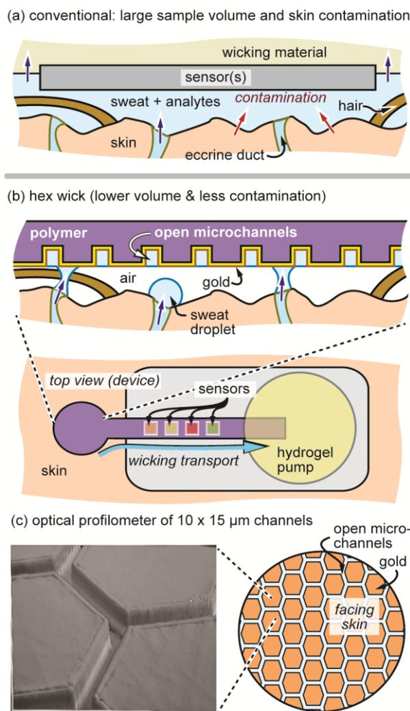
**Fig. 1** Approaches for sweat sampling **a**) conventional sensor-direct -on-skin with large sample volume with analyte contamination; **b**) hex wick (this work); **c**) optical profilometer image of 10x15 μm channels in the hex wick.
