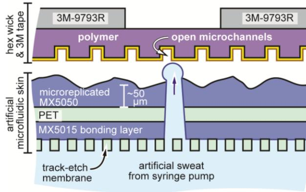
**Fig. 5** In-vitro artificial skin diagram of in-vitro test setup with artificial microfluidic skin.
