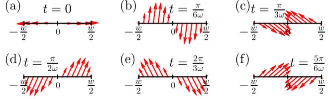
**Fig. 2** Plot of standing SAW displacement vectors along the interface of the channel and the piezoelectric substrate at  $z = 0$  at (a)  $t = 0$ , (b)  $t = \pi/6\omega$ , (c)  $t = \pi/3\omega$ , (d)  $t = \pi/2\omega$ , (e)  $t = 2\pi/3\omega$ , and (f)  $t = 5\pi/6\omega$ . The displacement function is obtained by superimposing two incoming traveling SAWs from the left and the right direction, see Eq. (11).
