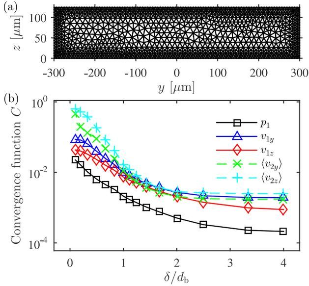
**Fig. 3** Mesh convergence analysis. (a) An illustrative computational mesh with 2478 triangular elements obtained with maximum element size near the boundary,  $d_b = 30\delta$ , while the maximum element size in the bulk of the domain was set to  $20\mu\text{m}$ . (b) Semi-logarithmic plot of the relative convergence parameter  $C$ , as given in Eq. (21), for decreasing mesh element size near the boundaries,  $d_b$ .
