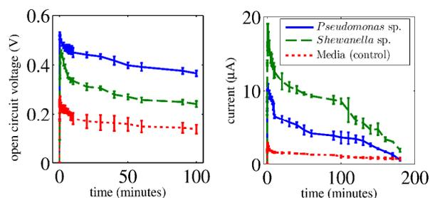
**Fig. 4** (a) Temporal variation of the open circuit voltage and (b) current for the paper MFC using both *P. aeruginosa*, *S. putrefaciens*, and control in an OTI mode.
