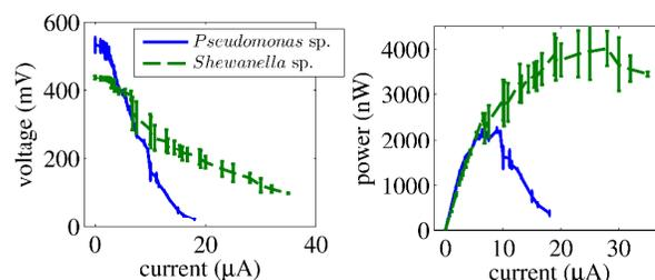
**Fig. 6** V-I and P-I characteristics of the device
