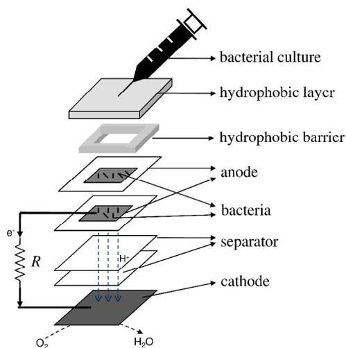
**Fig. 1** Schematic of the paper based bacterial fuel cell
