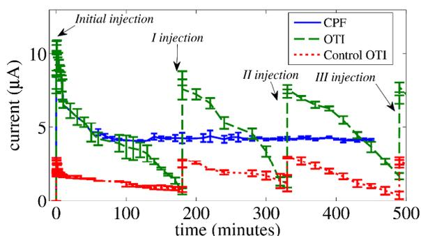
**Fig. 5** Demonstration of the two operating modes of the device under consideration. OTI stands for one time injection (with intermittent refill injections highlighted by the peaks occurring in Fig. 5) and CPF stands for Capillary flow mode. Both these modes were tried using *P.*
