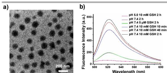
**Fig. 3** a) TEM images of FA-NP stained with uranyl acetate at pH 7.4. b) FITC fluorescence intensity changes of FA-NP in solutions of different pH and GSH concentrations. Only in the condition of pH 7.4 plus 10 mM GSH (cytosol-mimicking environment), the FITC fluorescence intensity increased obviously over time, indicating siRNA release. The polyplex FA-NP was formed at N/P=6.
