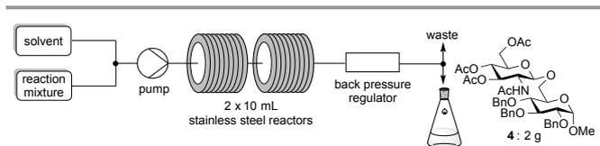
**Fig. 2** Flow system used for glycosylation reactions after optimization conditions.
