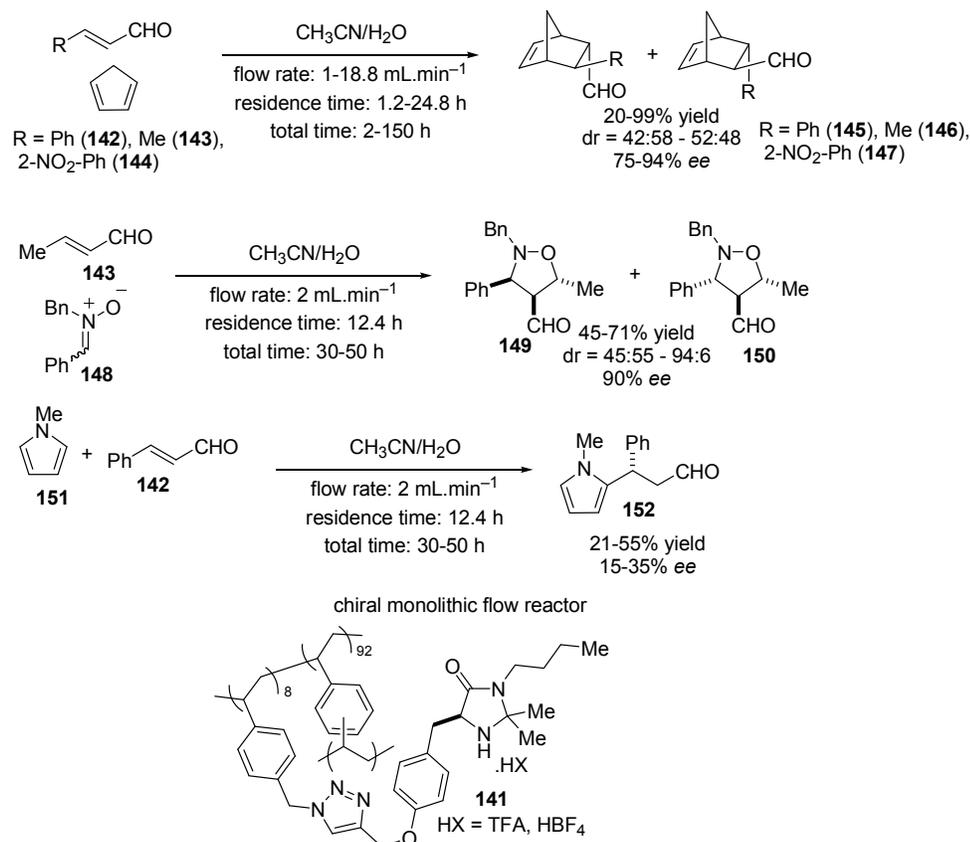
**Scheme 16:** Friedel-Crafts and cycloadditions reactions in a monolithic reactor loaded with a chiral imidazolone organocatalyst.
