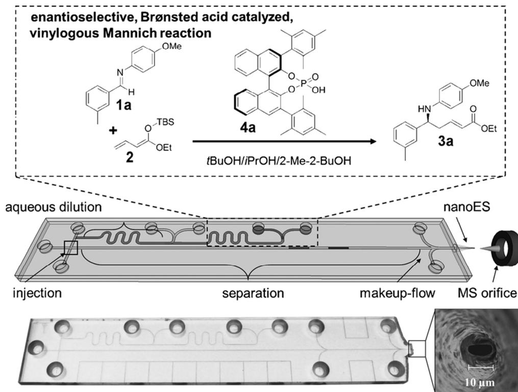
**Figure 1:** Designed microreactor for integrated analysis used on the bronsted acid organocatalyzed asymmetric vinylogous Mannich reaction.<sup>24</sup>
