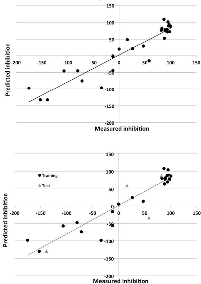
**Figure 5.** The observed versus predicted corrosion inhibition for 2024 alloy for the nonlinear model using DRAGON descriptors. Top panel: model for entire data set. Bottom panel: data set split into training (circles) and test (triangles) sets.
