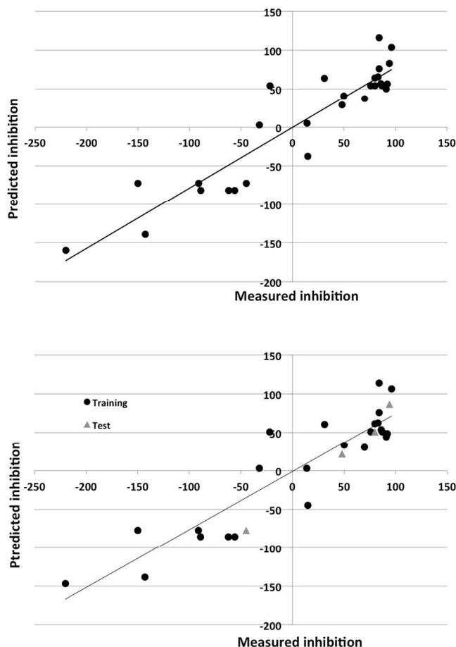
**Figure 4.** Observed versus predicted corrosion inhibition for 7075 alloy for the nonlinear models using the in-house intuitive descriptors. Top panel: model for entire data set. Bottom panel: data set split into training (circles) and test (triangles) sets.
