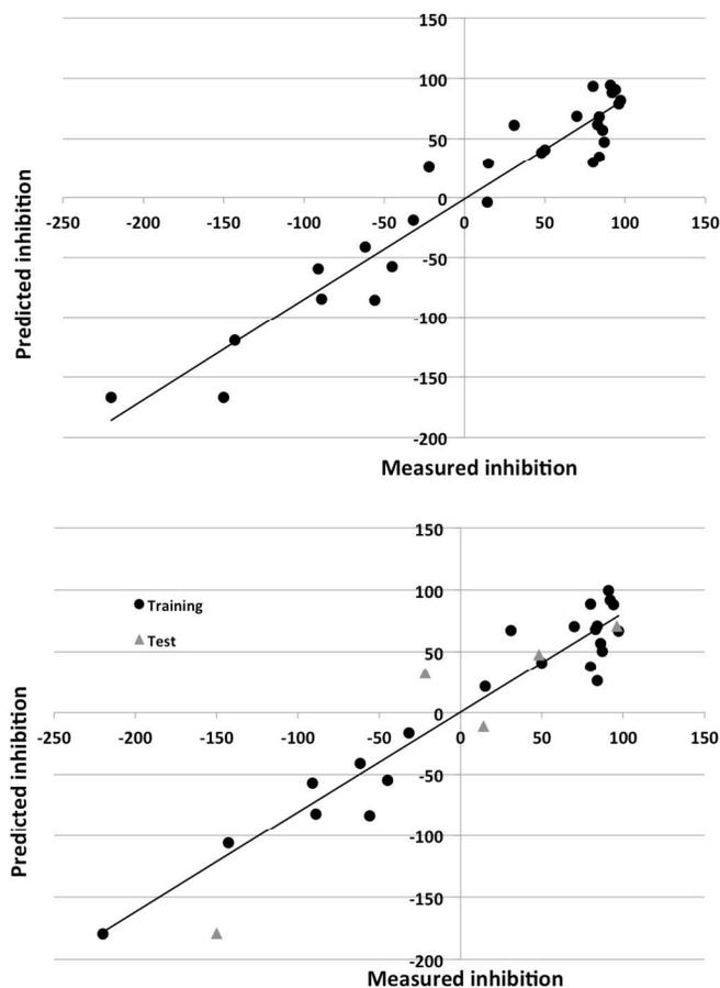
**Figure 3.** Observed versus predicted corrosion inhibition for 7075 alloy for the nonlinear model using DRAGON descriptors. Top panel: model for entire data set. Bottom panel: data set split into training (circles) and test (triangles) sets.
