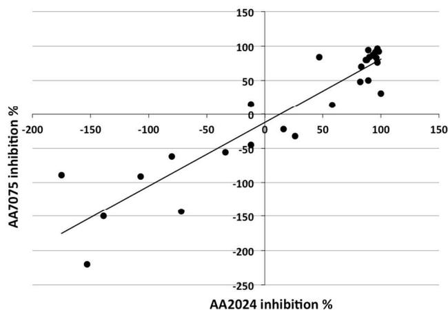
**Figure 2.** Correlation between corrosion inhibition on AA7075 and on AA2024 for 28 small organic inhibitors.
