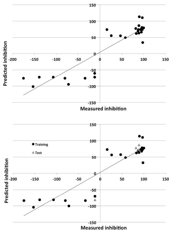
**Figure 6.** The observed versus predicted corrosion inhibition for 2024 alloy for the nonlinear models using the in-house intuitive descriptors. Top panel: model for entire data set. Bottom panel: data set split into training (circles) and test (triangles) sets.
