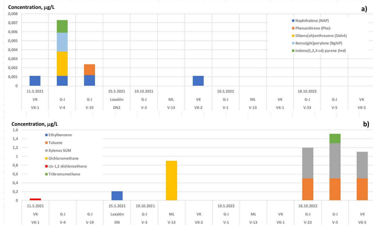
Fig. 2 PAHs (a) and VOCs (b) detected in samples from 11.5.2021 until 18.10.2022 (VK = Vatnsendakrikar, G-J = Gvendarbrunnar-Jadar, DN = distribution network, and ML = Myllulaekur).
