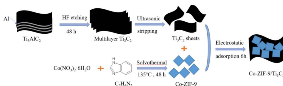
Fig. 9 Preparation process of Co-ZIF-9/ \text{Ti}_3\text{C}_2 composites. Reproduced from ref. 69 with permission from Wiley, copyright © 2022.
