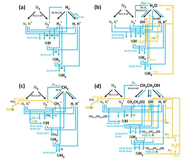
Fig. 3 Reaction diagrams of the  $N_2$  reduction processes in (a)  $N_2$ :  $H_2$ , (b)  $N_2 + H_2O$ , (c)  $N_2 + CH_4$ , (d) and  $N_2 + EtOH$  feedstocks. Black, blue, and yellow arrows indicate electron impact reactions, forward reactions, and reverse reactions, respectively.
