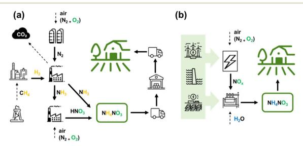
Fig. 1 Schematic representation of the fertilizer production and delivery chain for HB-based (a) and plasma-based (b)  $NH_4NO_3$ . The plasma-based route used as an example here involves electrocatalytic reduction as one step to directly obtain an aqueous solution of  $NH_4NO_3$ .
