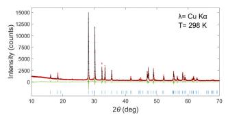
Fig. 2 Room-temperature PXRD pattern for M-TbTaO<sub>4</sub>: red dots, experimental data; black line, calculated intensities; green line, difference pattern; blue tick marks, Bragg reflection positions.
