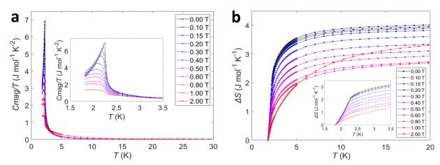
Fig. 5 (a) Magnetic heat capacity of M-TbTaO $_4$  as a function of temperature at selected fields and (b) magnetic entropy obtained by integration of  $C_{mag}/$ T. Inset: Data obtained at low temperatures.
