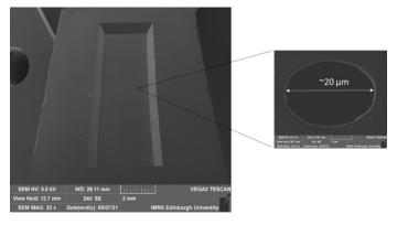
Fig. 3 SEM image of the back side of an MNE electrode showing the defined membrane and array area in the centre of the image. Also shown is a magnification of one of the micropores.
