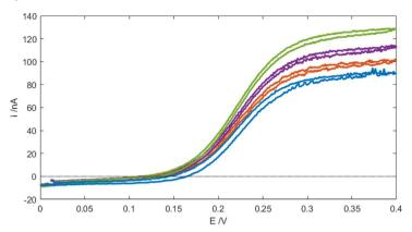
Fig. 5 Cyclic voltammograms (CVs) of 100  $\mu$ M FcMeOH in PBS at the MNE array at a scan rate of 100 mV s<sup>-1</sup> and flow rates  $V_{\rm f}=0$  (blue), 0.5 (red), 1 (purple), and 5 ml h<sup>-1</sup> (green). The initial direction of the scan is to more positive E.
