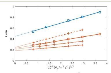
Fig. 12 Simulated currents at a single nanoband against  $V_f^{1/3}$  over the linear region with linear regression lines and extrapolated to zero flow. Simulations are for  $D=1.43\times 10^{-9}$  m<sup>2</sup> s<sup>-1</sup> (blue) and  $D=0.7\times 10^{-9}$  m<sup>2</sup> s<sup>-1</sup> (red) at  $x_{\rm E}=50$  nm (solid line, squares), and  $x_{\rm E}=10$  (dot-dash line), 25 (dotted line) and 100 nm (dashed line) for  $D=0.7\times 10^{-9}$  m<sup>2</sup> s<sup>-1</sup>.
