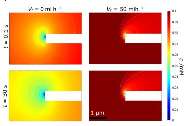
Fig. 11 Typical simulated concentration profiles showing the cross-section of the electrode for (left) region A,  $V_f = 0$  ml h<sup>-1</sup>, and (right) region B,  $V_f = 50$  ml h<sup>-1</sup>, at t = 0.1 (top) and 30 s (bottom). The white bar in the centre of each image shows the membrane with the FcMeOH depletion originating from the right-hand side of the nanoband. Flow is again from bottom to top in the right-hand images.
