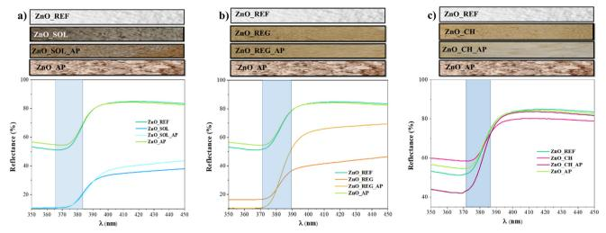
Fig. 3 Color changes and DR spectra of ZnO NPs before and after interaction with soil solutions, and after phenol degradation: a) ZnO\_SOL samples; b) ZnO\_REG samples; c) ZnO\_CH samples.
