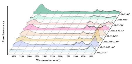
Fig. 4 IR spectra of ZnO NPs in the 1000–3700 cm<sup>-1</sup> region.
