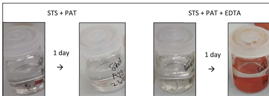
Fig. 4 Vials of \text{Sb}_2\text{S}_3 precursors sodium thiosulfate (STS) and potassium antimony tartrate (PAT) in water (left), and EDTA + STS + PAT in water (right), showing that upon addition of EDTA, a red powder forms over time in ambient conditions. Reproduced from ref. 59 with permission from Royal Society of Chemistry, copyright 2025.
