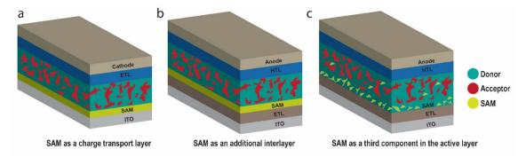
Fig. 2 (a–c) Schematic representation of the device architecture of organic solar cells employing self-assembled monolayer as a charge transport layer (represented as HTL in a normal device architecture), additional interlayer (represented as ETL modifier in an inverted device architecture), and third component (inverted device architecture) in a ternary blend system respectively.
