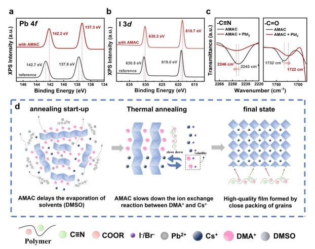
Fig. 3 (a) and (b) XPS spectra of Pb 4f and I 3d from perovskite films with and without AMAC incorporation. (c) FTIR spectra of AMAC and AMAC-PbI<sub>2</sub> films. (d) Schematic diagram of crystallization pathways of the perovskite with AMAC incorporation.
