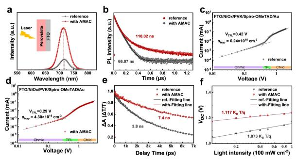
Fig. 5 (a) Steady-state PL spectra of perovskite films with and without AMAC incorporation. (b) TRPL spectra of perovskite films with and without AMAC incorporation. (c) and (d) SCLC measurements without and with AMAC incorporation, devices structure: FTO/NiOx/perovskite/Spiro-OMeTAD/Au. (e) Dynamic evolution of the bleaching recovery from measuring F-TAS. (f) V<sub>OC</sub> variation with light intensity.
