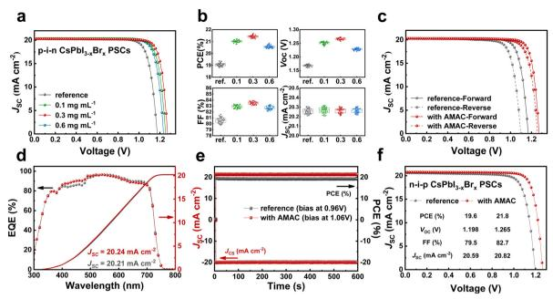
Fig. 4 (a) J-V characterization of p-i-n CsPbl<sub>3-x</sub>Br<sub>x</sub> PSCs incorporated with different amounts of AMAC under 100 mW cm<sup>-2</sup> illumination (the active area is 0.09 cm<sup>2</sup>). (b) Statistical box charts of PV parameters. (c) Hysteresis with and without AMAC-incorporated PSCs. (d) EQE and integrated  $J_{SC}$ . (e) SPO at MPP tracking. (f) J-V characterization of n-i-p CsPbl<sub>3-x</sub>Br<sub>x</sub> PSCs with and without AMAC incorporation.
