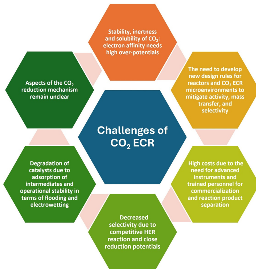
Scheme 1 Challenges during the ECR of \text{CO}_2 .
