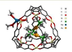
Fig. 5 X-ray crystal structure of **GG@H**. For the sake of clarity, hydrogen atoms of  $\mathbf{H}$ , the *n*-octyl chains at Si and three Na(MeOH)<sub>3</sub><sup>+</sup> are omitted.
