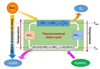
**Fig. 1** Principle of two-step thermochemical cycling for solar fuel production based on ceria-based redox materials. Reproduced with permission<sup>11</sup> Copyright 2023, Elsevier.
